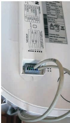
Mount the Electronic Driver inside the Split AC unit, if there is a space constraint then mount it outside the indoor AC unit as shown, the AC input is to be given to the AC side mark of the driver circuit and the output side is to be connected to the UVC light wires.
